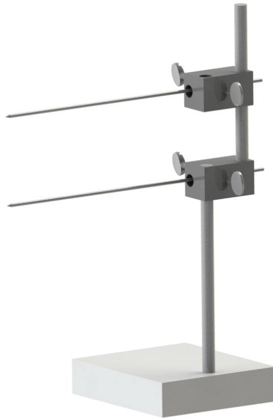
Figure 2.5: Ulnar support tower with two pins to rigidly fix the ulna to the simulator base; refer to Figure 2.1 for the orientation of the ulnar support with respect to the arm
